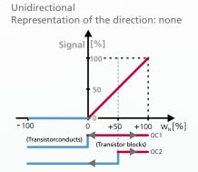
Remark: in an unidirectional design, the switching output OC1 is used as flow indicator by default (configurable). It will clearly show a flow higher than 0 m/s by blocking and will switch if this is less or equal to 0 m/s. Arrows in the representation of the switching outputs mean that the threshold value can be configurated. The factory setting for the switching output OC2 is 50 % of the measurement range (option: customer-specific switch point).
