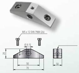
Wall mounting bracket item no. 503 895 For mounting in front of wall openings Material: Anodized aluminum
