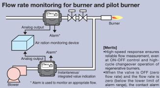
signal can be set to no output. •Timing (1 to 30s) can be set for judging whether or not the increase in flow rate above the alarm setpoint is an actual condition for an alarm signal. Since momentary flow fluctuations can generate alarm signals, this function can prevent false alarms.
