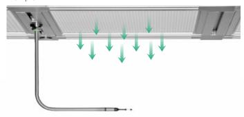
SS 20.515 LED (angular; 270 mm x 300 mm), installation to the ceiling below a laminar flow unit (with a type 1 fixation)
