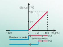
Remark: In an unidirectional design, the switching output OC1 is used as flow indicator by default (configurable). It will clearly show a flow higher than 0 m/s by blocking and will switch if this is less or equal to 0 m/s. Arrows in the representation of the switching outputs mean that the threshold value can be configured. The factory setting for the switching output OC2 is 50 % of the measurement range (option: customer-specific switch point).
