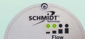
The LED display is dual function. In 'normal' operation the 4 x LEDs illuminate steady green in sequence. In 'fault' condition reportable faults are indicated by red flashing LEDs. The instrument will output V and mA and change-over is automatic.
